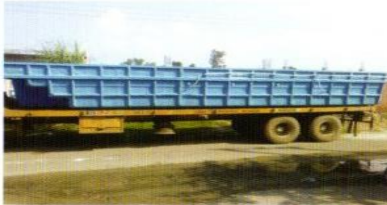
2. Transportation of swimming pool on Truck.
